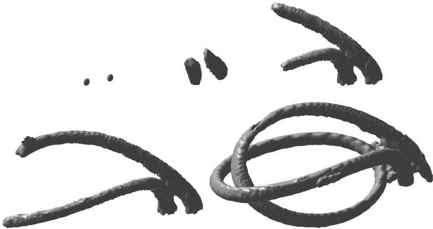
Fig. 7. Image sequence of an evolving surface, going from left to right and top to bottom, segmenting a flow phantom by using both velocity and intensity information. The surface is initialized as two spheres (top left)
