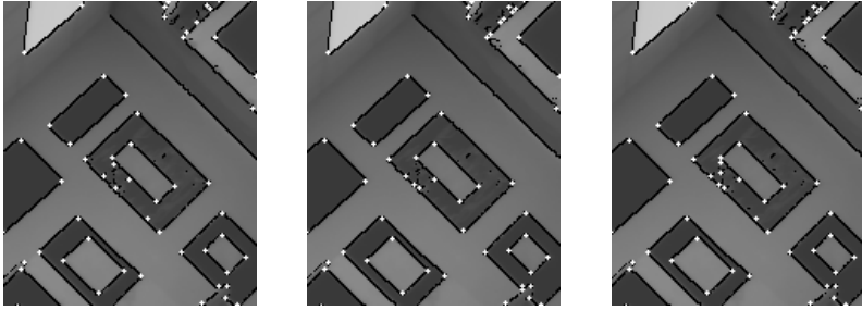
Fig. 5. Integrated boundary detection from boundary tensor, GET operator ( \sigma_3/\sigma_1 = 1.5 ) and GET operator (Scharrr filter)
