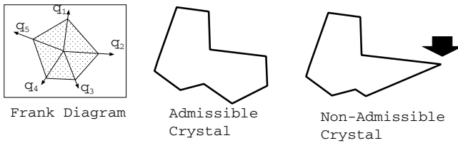
Fig. 2. The Wulff shape, an admissible crystal, and a non-admissible crystal. At the vertex indicated by the arrow, the condition is not satisfied
