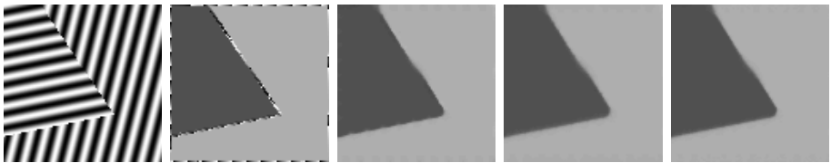
Fig. 2. Left to right: (a) Synthetic image with oriented textures, inspired by [16]. (b) Local orientations computed via DoGs and visualised as grey-values. (c) Orientations after median filtering of the orientation matrices with Frobenius norm and a disk-shaped structure element of diameter 7. (d) Same with structure element of diameter 9. (e) Spectral norm median filtering, diameter 9
