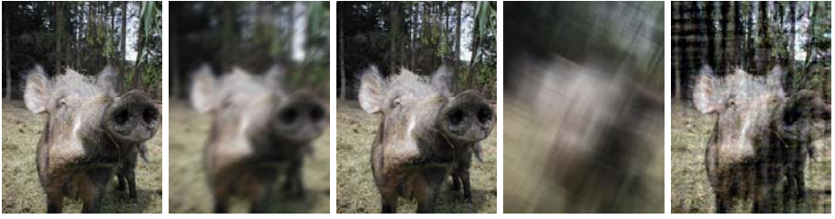
Fig. 2. Left to right: Photograph, 480 \times 640 pixels. – Blurred with banana-shaped kernel. – Deblurred by diffusion–reaction method with Perona–Malik diffusivity, \lambda = 5 , \alpha = 0.001 , 1000 iterations. – Photograph blurred with discontinuous kernel. – Deblurred by diffusion–reaction method with Perona–Malik diffusivity, \lambda = 1 ; the continuation strategy was used with two steps for the diffusion weight: 2400 iterations with \alpha = 0.01 followed by 2400 iterations with \alpha = 0
