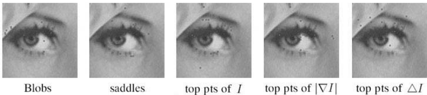
Fig. 1. Examples of the different points used for reconstruction, projected on the lena64 image. From left to right: Blobs, scale space saddles, top points of image I , top points of |\nabla I| and top points of \Delta I . For all feature points, the 19 strongest (relative to their respective feature strength) points are shown
